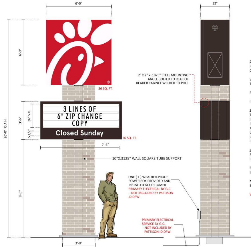
OPTION 2 A D/F PYLON WITH READERBOARD SIGN SCALE: 3/8" = 1'-0" ONE (1) REQUIRED - MANUFACTURE AND INSTALL 62 SF
