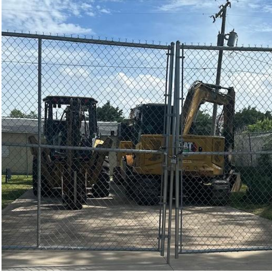
Rubber-tire backhoe loader and mini excavator
